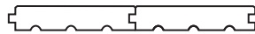
T+G: MICRO BEVEL Standard on most engineered products, recommended for most pre-finished items & wall cladding
