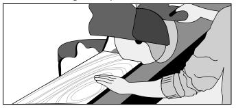
Using a chop saw, cut your ThinClad cladding to fit your space. You may be abe to start with full length boards as delivered from Anthology Woods. Stagger the vertical seams between courses by at least 12". Ideally these joints land on a framing member for secure fastening.
