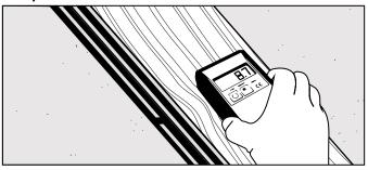
Inspect your order for any damage and report on the BOL prior to accepting the shipment. Perform a moisture check of your cladding and substrate. The wood needs to be properly acclimated to the space. There should be no more than a 2-3% moisture difference between substrate and the Thinclad product.
